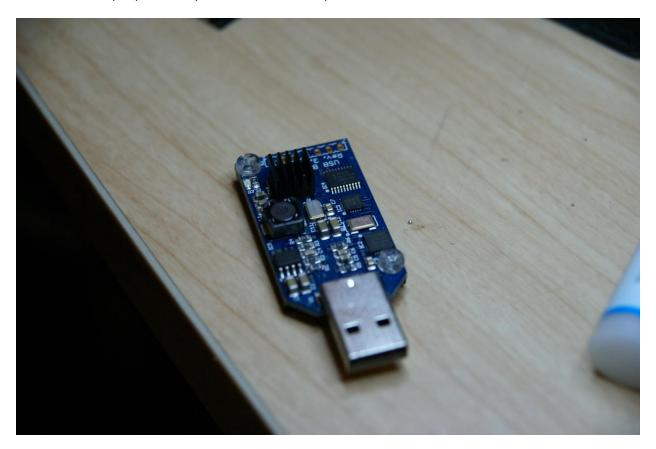
Lastly, reinstall the thermal pad and heat spreader back on your board after about 5 min of cooling. Reinstall them simply by reversing the steps that I showed earlier. Plug your eruptor back in and start your favorite mining program; and if all is well, you should see something like this:
